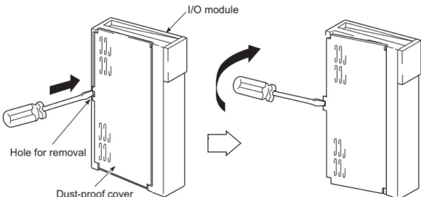
As for removing the dustproof cover, insert the tip of a flathead screwdriver into the removal hole, and then tilt the screwdriver to pry the cover off, as shown in the figure.
